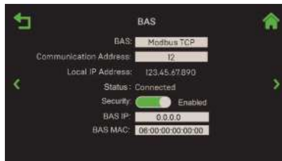
Figure 1.2: Modbus TCP Security Screen
