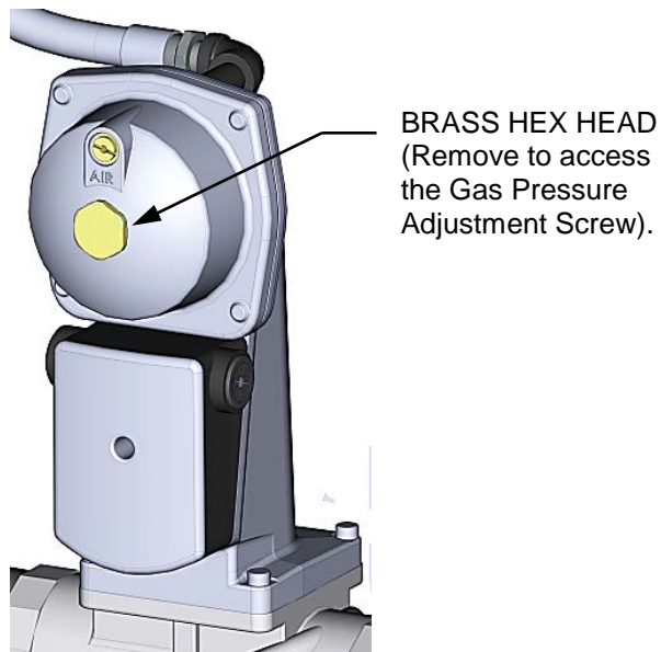
Figure 4-3: Gas Pressure Adjustment Screw Location
