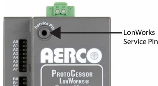
Figure 4-5: LonWorks Service Pin Location
