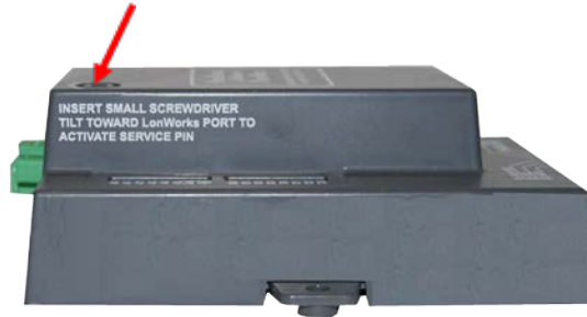
Figure 4-6: LonWorks Service Pin Location
