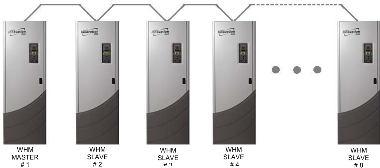
Figure 8-3. Typical Daisy-Chain Modbus/RS485 Network
