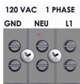
Figure 2-10. AC Terminal Block Configurations
