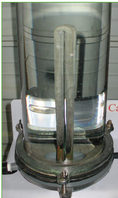
Untreated Scale build-up in untreated water
